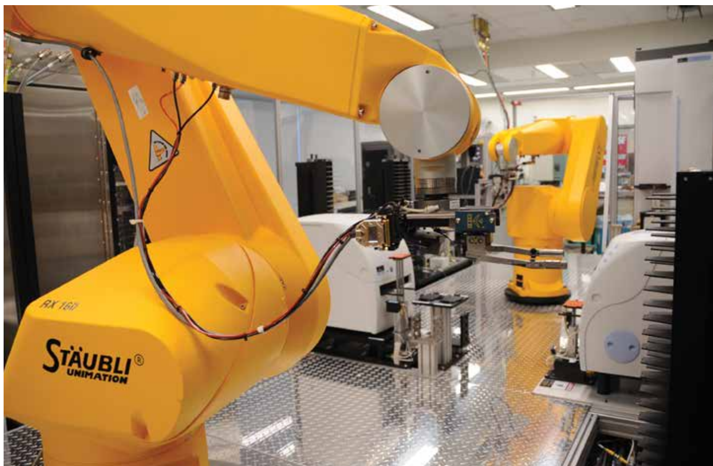
FIG. 2. A robotic arm retrieves well plates for analysis in a high-throughput screening contract lab maintained by the National Institutes of Health in Bethesda, Maryland, USA. Source: https://ncats.nih.gov
