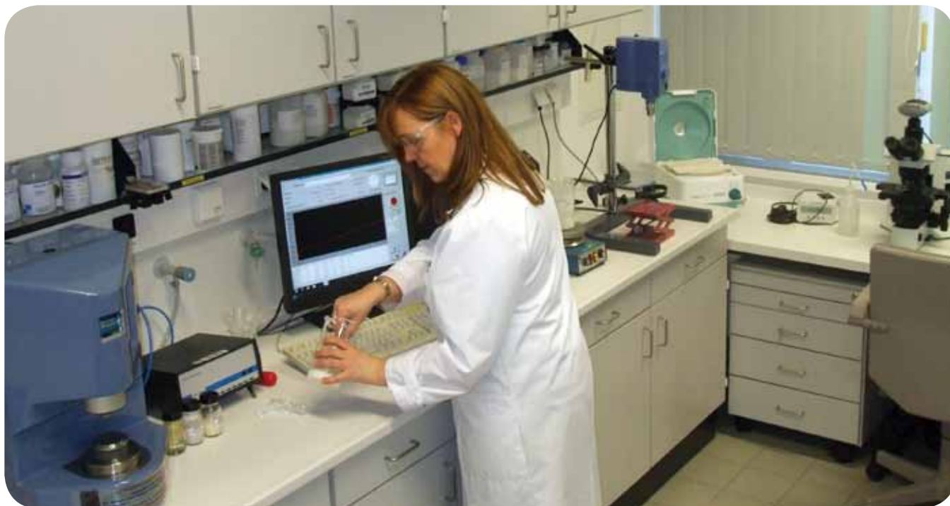
FIG. 1. A researcher in a cosmetics laboratory uses a rheometer to measure the flow properties of a formulation. Courtesy of Azelis, Moers, Germany.
