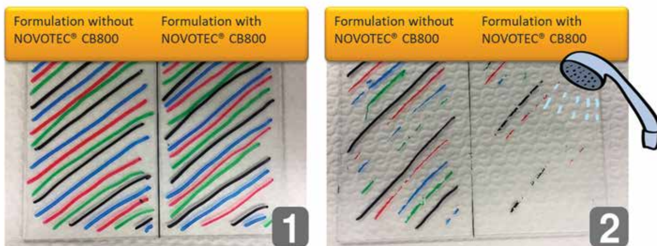
FIG. 2. Comparison of a surface coated with and without NOVOTEC® before (1) and after (2) cleaning. Source: Gelita.
