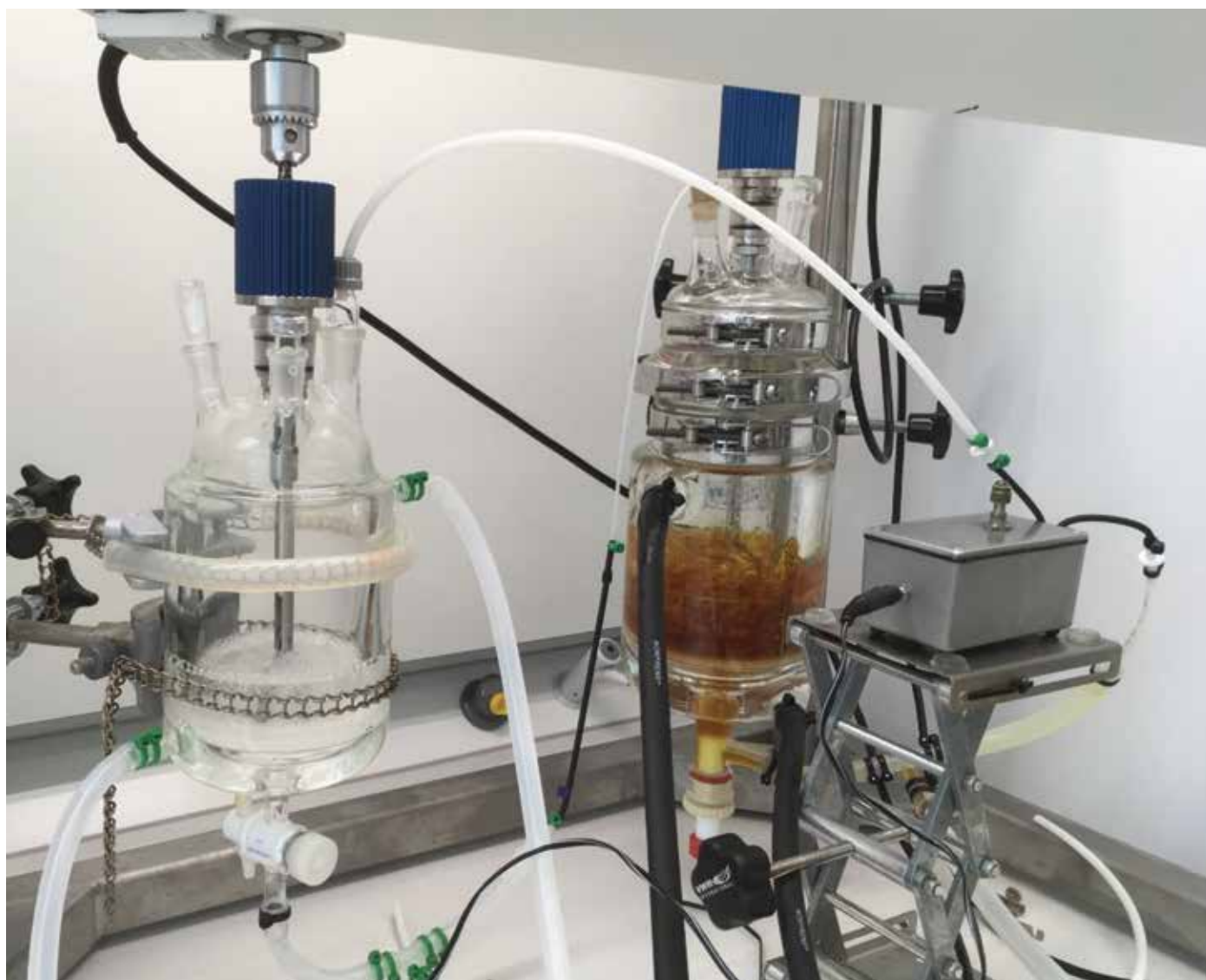
FIG. 1. Stirred bubble reactor setup in laboratory. A vacuum pump circulates methanol vapor from condenser tank to the reactor. Water from the reactor is brought to the condenser.
